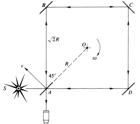
Interferometer rotates with angular velocity  $\omega$
