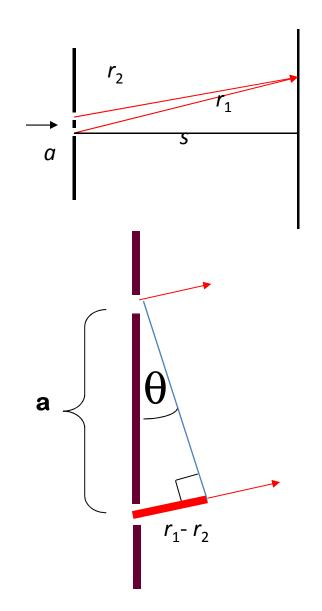
Far from the source,  $s \gg a$ ,  $I = 4I_0 \cos^2 \frac{\delta}{2}$  $=4I_0\cos^2\left(\frac{k(r_1-r_2)}{2}\right)$  $r_1 - r_2 = a \sin \theta \approx a \tan \theta \approx \frac{ay}{a}$  $I \approx 4I_0 \cos^2 \frac{kay}{2s} = 4I_0 \cos^2 \frac{\pi ay}{s\lambda}$
