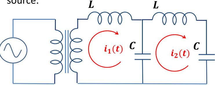
• Resonance would occur at the frequency of each normal mode:  $(3 + \sqrt{5})$
