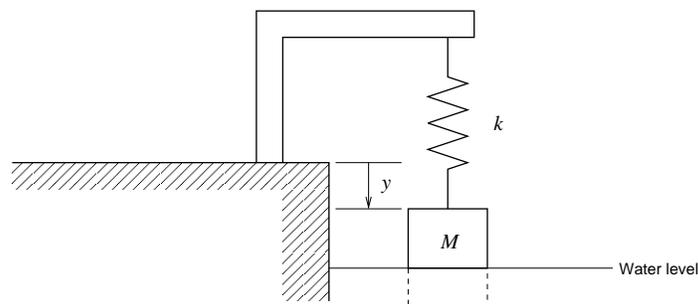
The cylinder has a total mass,  $M$ , and a cross sectional area  $A$  and the water, which has density  $\rho$ , provides an upward buoyant force on the cylinder. You can assume that some part of the cylinder always remains under water and that the cylinder is never completely submerged. Suppose that the distance  $y$ , as shown on the diagram, has a value of  $y = 0$  when the mass is in a state of static equilibrium.
