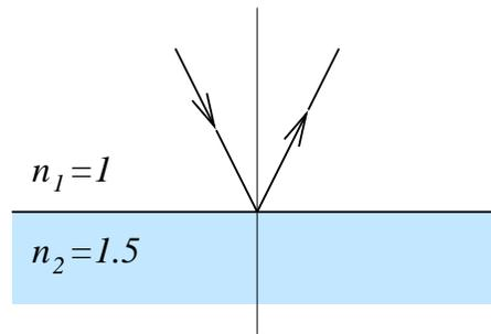
(b) Calculate the effective reflection coefficients,  $R'_{\perp}$  and  $R'_{\parallel}$ , that account for light reflected from both front and back surfaces of the material, as shown below. (In this example we assume that the light reflected from the front and back surfaces adds incoherently.)
