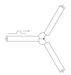
(a) The power carried by a pulse with current I is given by  $P = ZI^2$ . Given that the current would be split equally between the two transmission lines on the right, what is the effective impedance of this *pair* of transmission lines? (b) If a pulse, incident from the left as shown, has an amplitude of  $V_i$ , what is the amplitude of the pulse that is reflected from the point at which the transmission lines are connected? Is the pulse inverted?
