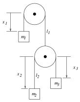
in which the strings have length  $l_1$  and  $l_2$  and the pulleys are assumed to be massless.
