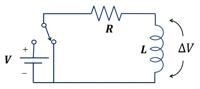
The current can still flow after the switch is flipped but now the voltage source isn't adding energy to the circuit.
