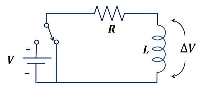
• What is the potential difference across the inductor after the switch is opened?  $\Delta V = 0.632 V$
