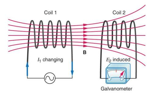
• In this case the flux through coil 2 is proportional to the current through coil 1.
