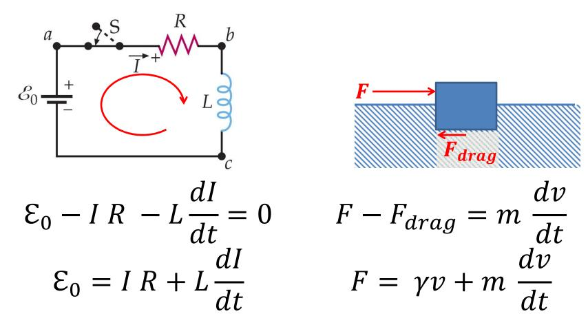
The mechanical analog of inductance is mass. The inertia associated with a mass resists changes in velocity. The inductance resists changes in current.
