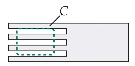
Slots cut into metal break the loop into smaller pieces...
