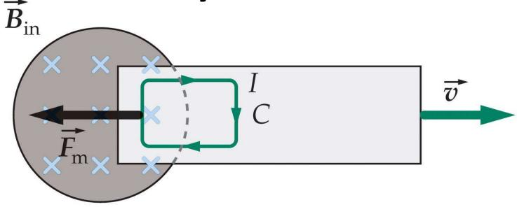
Relative motion between magnetic field and conductor induces a current in the conductor.
