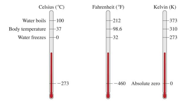
The bulb and part of the tube are filled with a red liquid that expands predictably when heated and that shrinks when cooled.
