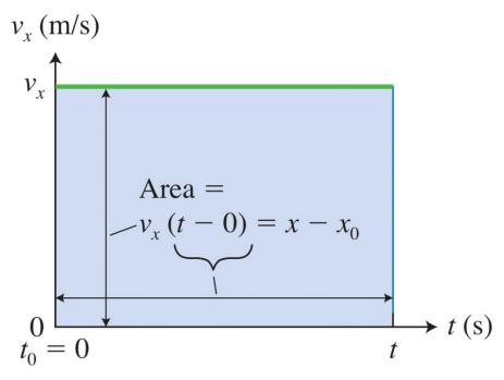
An object's displacement  $x - x_0$  between  $t_0 = 0$  and time t is the area between the  $v_x$ -versus-t curve and the t axis.
