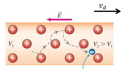
In the presence of an electric field, the electrons drift toward the higher *V* region.
