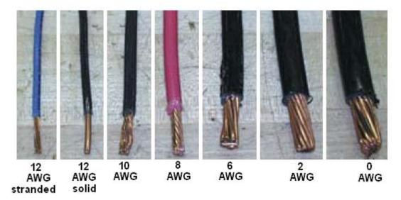
Determine the resistance of a 100 meter length of 12 AWG (2.052 mm diameter) sold wire made of the following materials:
