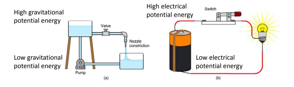
Resistance to flow: the ratio of the potential energy difference to the current flowing.
