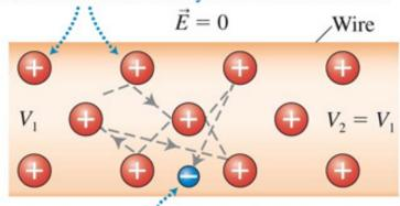
In the absence of an electric field, the electrons move randomly within the wire.
