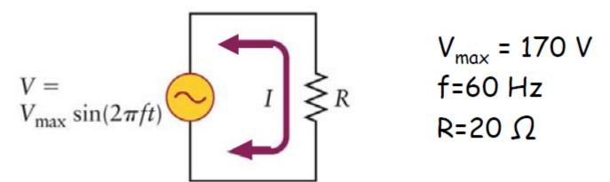
What are  $V_{rms}$ ,  $I_{rms}$ , and average power dissipated in load? What are  $V_{max}$ ,  $I_{max}$ , and maximum power dissipated in load?
