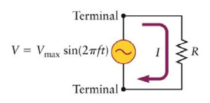
Ohm's Law: I = V/R  $V(t) = V_{max} \sin(2\pi f t)$   $I(t) = I_{max} \sin(2\pi f t)$  $I_{max} = V_{max}/R$
