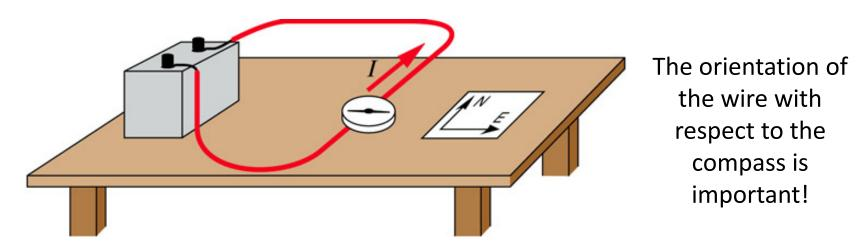
The current through the wire caused a deflection in the nearby compass needle.
