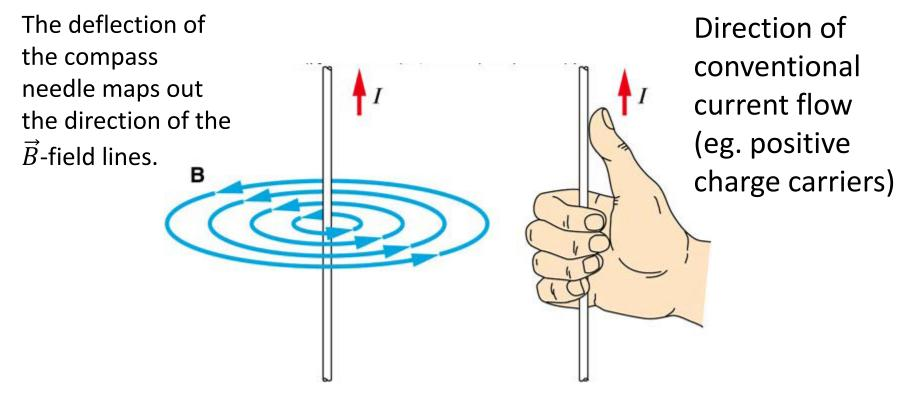
This particular version of "the right-hand rule" shows how to get the direction of the magnetic field right.
