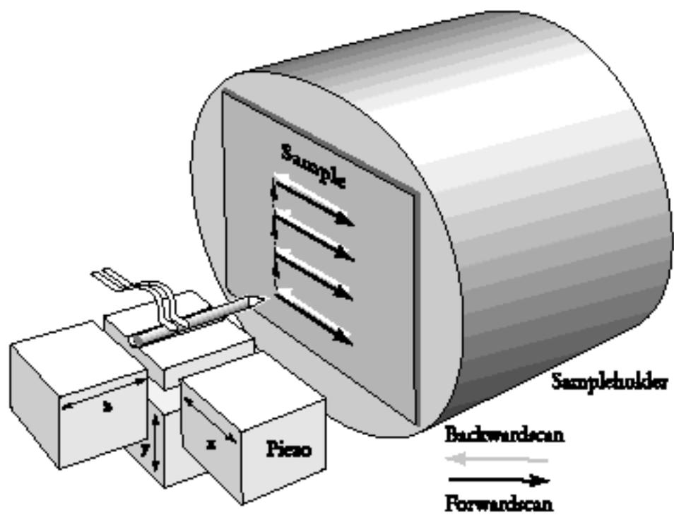
Figure 1. Tip configuration on an STM system<sup>[2]</sup>.
