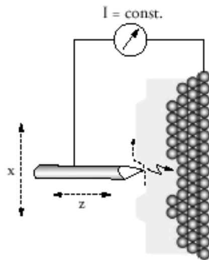
Figure 2. The probing tip while scanning<sup>[2]</sup>.
