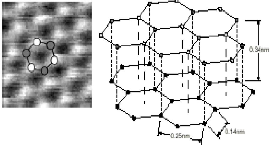
Figure 7. Lattice structure of graphite<sup>[2]</sup>.
