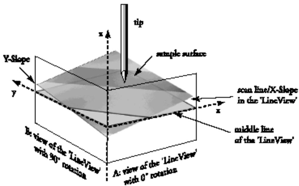
Figure 3. Sample orientation before tilt adjustments<sup>[2]</sup>.
