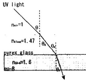
Figure 5: Schematic view of UV light pass through air, glass and SU-8
