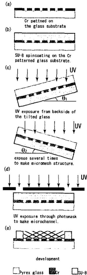
Figure 1: Fabrication process of an in-channel 3-D micromesh structure
