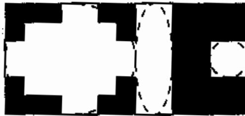
Figure 4: Pipes of elliptical cross-section are fitted within the pore-space of each fracture along rows perpendicular to the flow direction.
