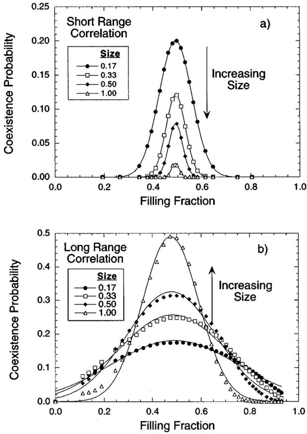
FIG. 2. The coexistence probabilities for (a)  $T=1$  (short-range correlations),  $N=10\,000$ , and  $b=75$ ; and (b)  $T=5$  (long-range correlations),  $N=10$ , and  $b=2.37$  as functions of observation size. The coexistence probability decreases with increasing size for short-range correlations, but increases with increasing size for long-range correlations.
