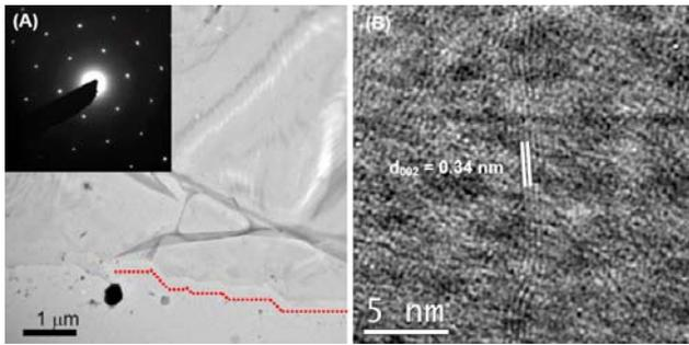
**Figure 1:** TEM images of graphene. (a) Low magnification image with step shaped edges, highlighted by red dash lines. Inset shows the SAED pattern of the graphene film. (b) HRTEM image of wrinkles in the graphene film, apparently of 3–4 layers.
