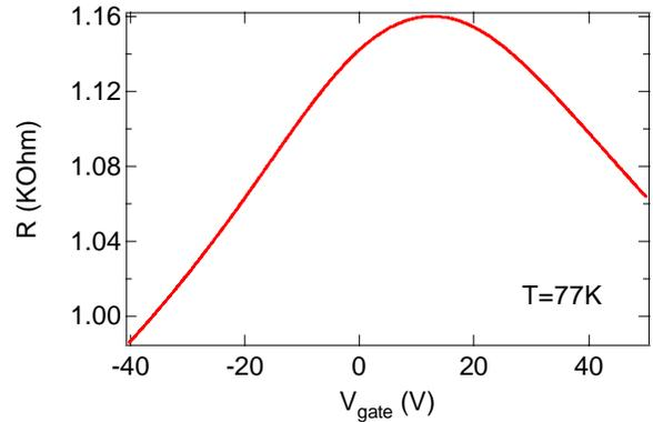
**Figure 3:** Four-terminal resistance as a function of back gate voltage  $V_{\text{gate}}$ , showing the electric field effect.
