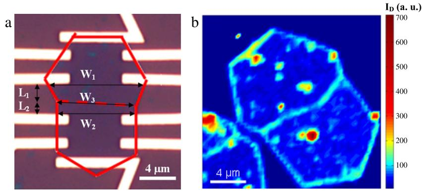
**Fig. 1.** (a) Optical image of multi-terminal device on two merged graphene grains. (b) Raman mapping of the  $D$  band intensity ( $I_D$ ) for the sample depicted in (a) prior to the device fabrication.
