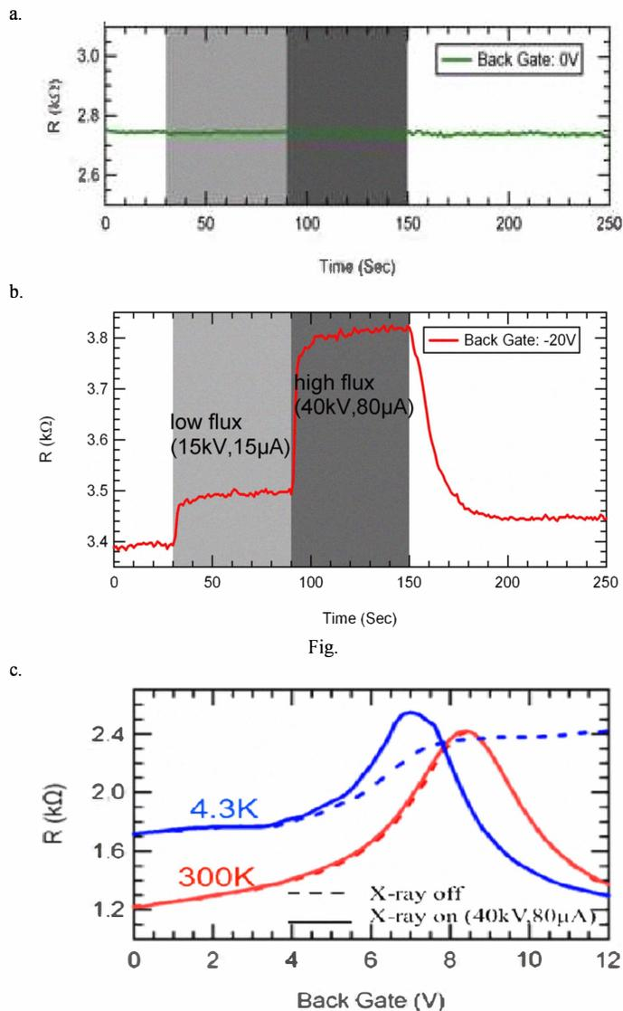
Fig. 3. a. Demonstration of proof of concept: Field effect is what causes a change in graphene resistance [4]; b. GFET response to low (15 keV, 15  $\mu$ A) and high (40 keV, 80  $\mu$ A) X-ray flux [4]; c. response of Si-based GFET at 4.3K and 300K [4]
