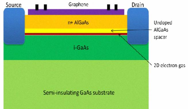
Fig. 8. Graphene on AlGaAs/GaAs HEMT
