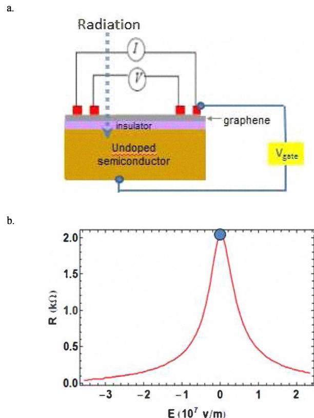
Fig. 1. a. A prototype graphene field effect transistor (GFET); b. graphene exhibits a sharp change in resistance as a function of applied field, near the charge neutrality point (“Dirac point”). Data shown are measured in a representative GFET with doped Si as substrate and 300nm-thick SiO<sub>2</sub> as buffer layer at room temperature [4].
