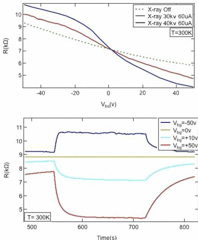
Fig. 5. Response of SiC based GFET to X-rays at 300 K
