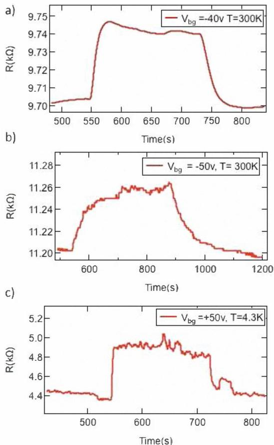
Fig. 6 Typical response of SiC-based GFET to a) light photons, b) gamma rays. Also shown in c) is the response of a GaAs-based GFET to X-rays.
