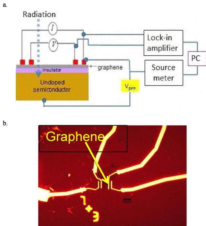
Fig. 2. a. Experimental schematic for X-ray irradiation on GFET and four-probe measurement with graphene [4]; 2b. Optical microscope image of a graphene device with 4 metal electrodes.
