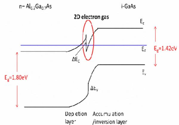
Fig. 9. Band diagram of AlGaAs/GaAs heterojunction
