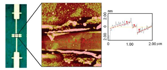
**Figure 2.** (a) Au electrodes are deposited by electron beam lithography on top of chemically reduced graphite oxide to form a transistor as imaged by an optical microscope. (b) The graphene sheets appear as thin platelets between the somewhat grainy gold electrodes as imaged by AFM. (c) When the AFM tip in tapping mode is moved across the graphene surface (red dotted line in b) steps of 8-9 Å are observed (red arrows).
