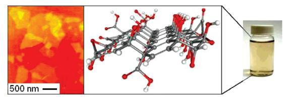
**Figure 1.** (a) An AFM image of GO platelets after deposition onto a Si wafer with a 300 nm SiO<sub>2</sub> epitaxial coating. (b) A three-dimensional molecular model of graphite oxide (GO) showing a puckered carbon sheet with -OH and -COOH functional groups (carbon = gray, oxygen = red, hydrogen = white). (c) A GO dispersion in water.
