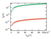
**Figure 3.** Current  $(I_d)$ -voltage  $(V_{ds})$  plots taken on graphite oxide films before  $(\bigcirc)$  and after  $(\times)$  reduction reveal a 10000-fold decrease in sheet resistance.
