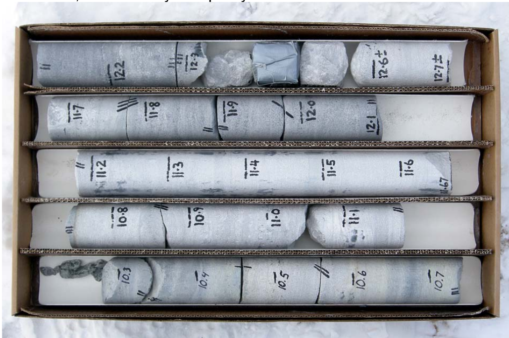
Sandstone core interval from 10.3 – 12.7 meters.
