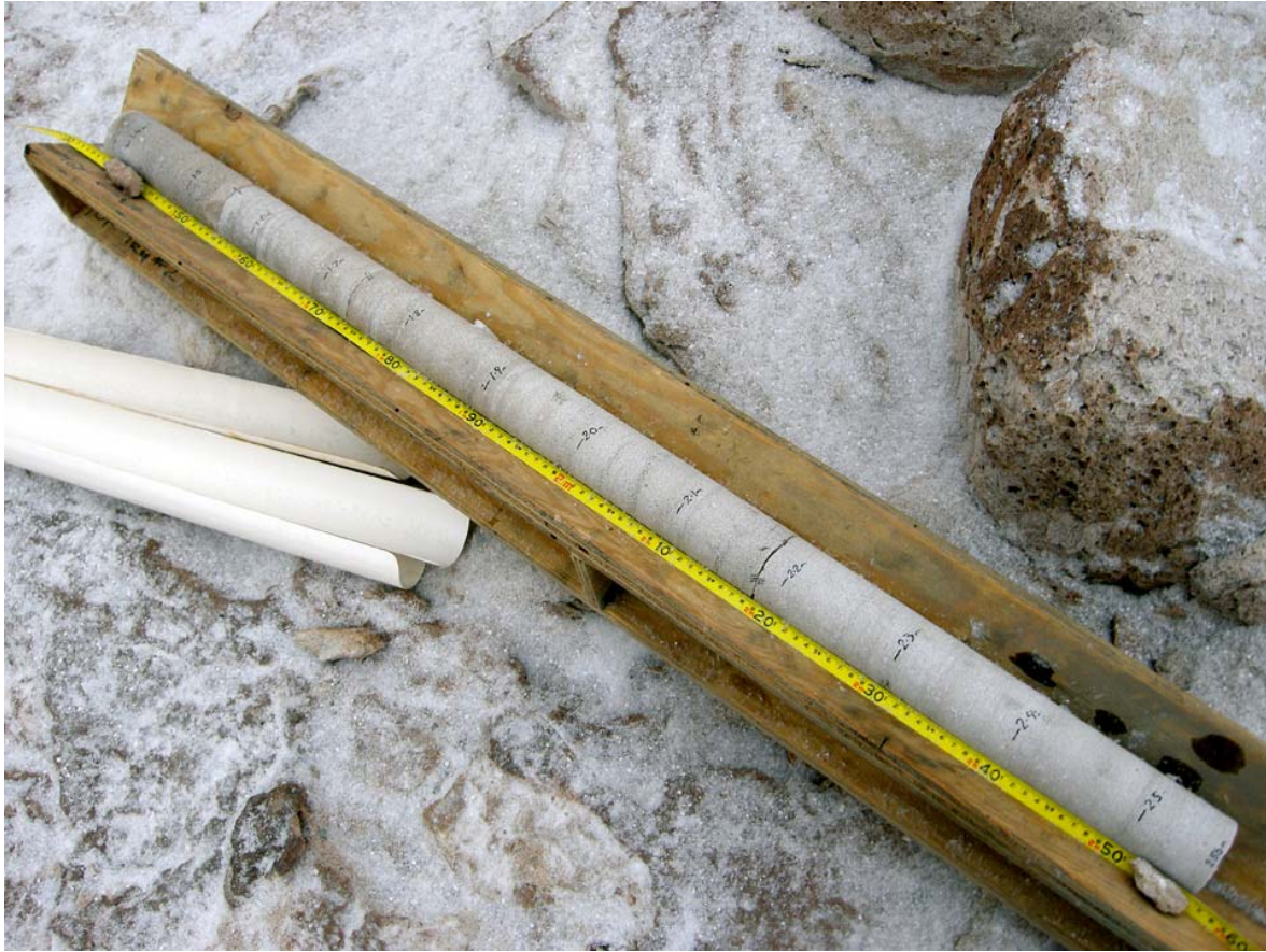
Quartz sandstone core from 1.4 – 2.6 meters. Recovery was close to 100% in the top 5 meters of the hole, as shown by the quality of the core here.
