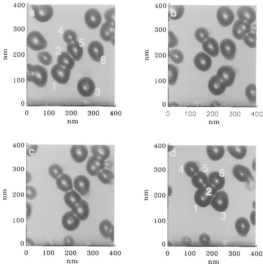
FIG. 2. (a) Initial noncontact image of Au clusters on a WSe<sub>2</sub> substrate. In (b)–(d), sequential noncontact images are shown after the AFM tip was used to reposition a number of different clusters on the substrate. The grayscale used in this figure was generated by an algorithm using an artificial light source designed to highlight the cluster location. For this reason, no height information is contained in the grayscale as is the usual case.
