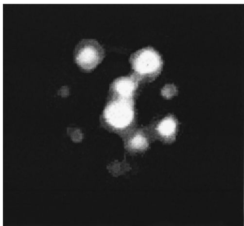
FIG. 4. A field-ion image from a \sim 1.5 nm Au cluster, annealed before deposition at a temperature of 1200 K, cooled to 300 K, and landed on a W tip. The imaging gas is Ar and the temperature of the tip and cluster is 100 K.
