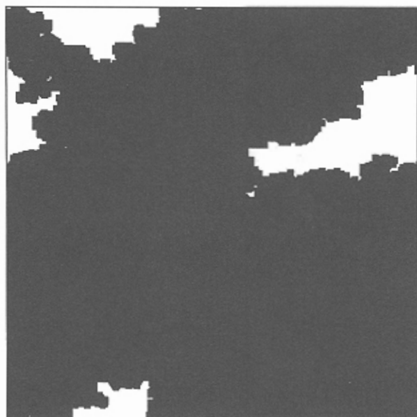
Figure 1. Stratified continuum percolation model of flow paths (black regions) in a fracture for five tiers, twelve points per tier, and a scale factor of 2.37. White regions represent areas of contact.
