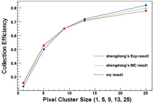
PIXEL cluster size: the number of PIXEL summed with the hit PIXEL as center (e.g. 5 x 5 PIXEL array is a cluster of 25 PIXELs)
