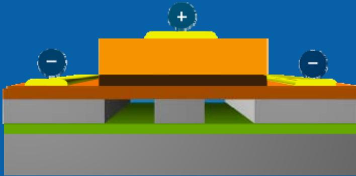
5) The Indium phosphide is etched and electrical contacts are added
