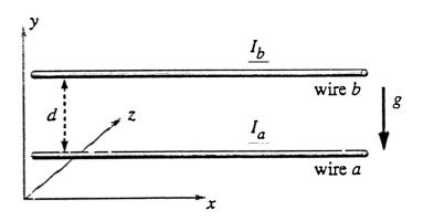
Wire b is displaced from position d by a small distance  $\Delta y$  and released. Show that it undergoes simple harmonic motion with the same frequency as a simple pendulum of length d. The acceleration of gravity is in the -y direction and is given by the constant g.
