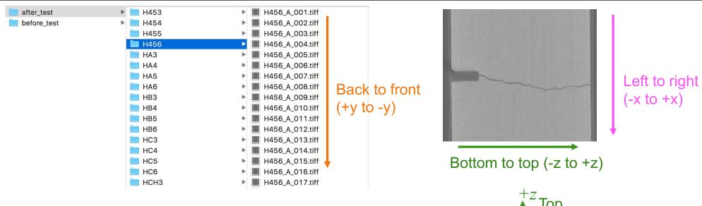
Notch area was scanned before and after the test.
