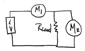
When connecting amp-meters or volt-meters in a circuit which is the correct way to measure the current and voltage in the load?
