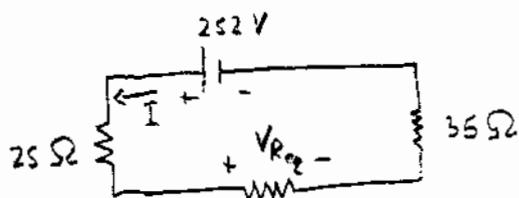
$$R_{eq} = \frac{1}{\frac{1}{36} + \frac{1}{18}} = \frac{1}{\frac{1+2}{36}} = \frac{36}{3} = 12\Omega$$
