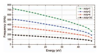
FIG. 3. Calculated bounce frequencies in the anharmonic potential well used for the experiments, of particles with mass-to-charge ratios 1 (green-squares), 2 (blue-circles), 4 (red-triangles), and 14 (black-diamonds), in units of proton mass/fundamental charge  $(m_p/e)$ . Here, and in what follows, the energy is chosen to be zero at the potential well minimum.
