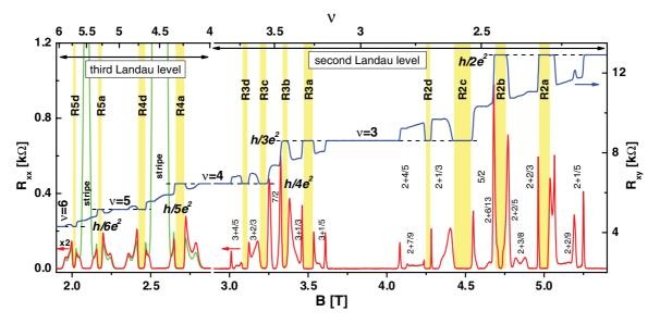
FIG. 1. (Color online) The magnetoresistance in the second  $(2 < \nu < 4)$  and third  $(4 < \nu < 6)$  Landau levels. Both the longitudinal  $(R_{xx})$  and the Hall  $(R_{xy})$  resistances are measured at 77 mK in the TLL and at 6.9 mK in the SLL. RIQHSs are marked by shaded stripes and FQHSs by their filling factors. In the TLL the two  $R_{xx}$  traces shown are measured along mutually perpendicular directions and, for clarity, are magnified by a factor of 2.
