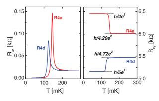
FIG. 3. (Color online) The magnetoresistance  $R_{xx}$  and the Hall resistance  $R_{xy}$  of two RIQHSs in the third Landau level measured at v = 4.29 and v = 4.72.
